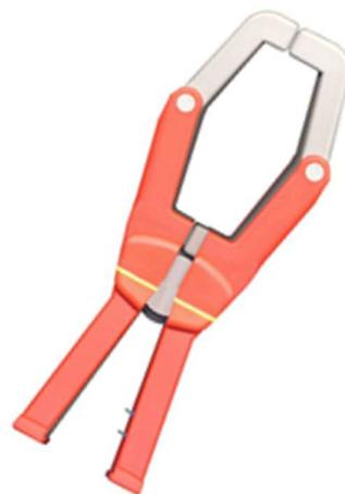
The H50.3C 2000A - 5000A/2V current probe has been designed for use with multimeters, recorders, power analysers, safety testers etc. for accurate non intrusive measurement of AC/DC current. Using Hall effect technology, the H50.3C 2000A - 5000A/2V can measure currents from 20 A to 5000 A over a frequency range of DC to 1kHz.
